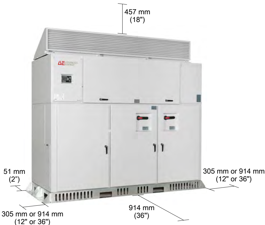
Figure 3-1. Inverter clearances
