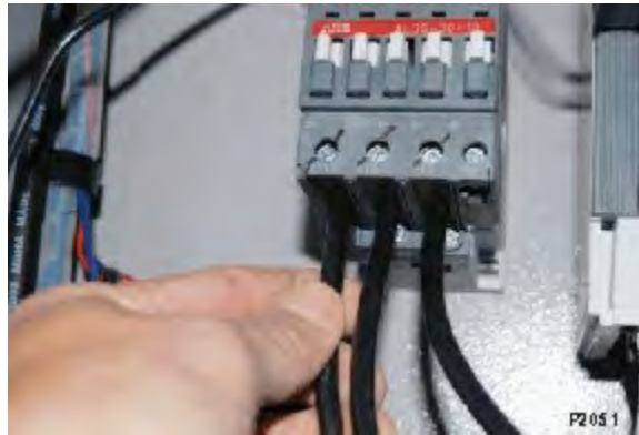
Figure 4-6. Pull-test of cable screw terminal connection
