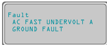
Figure 5-11. Ground fault error message
